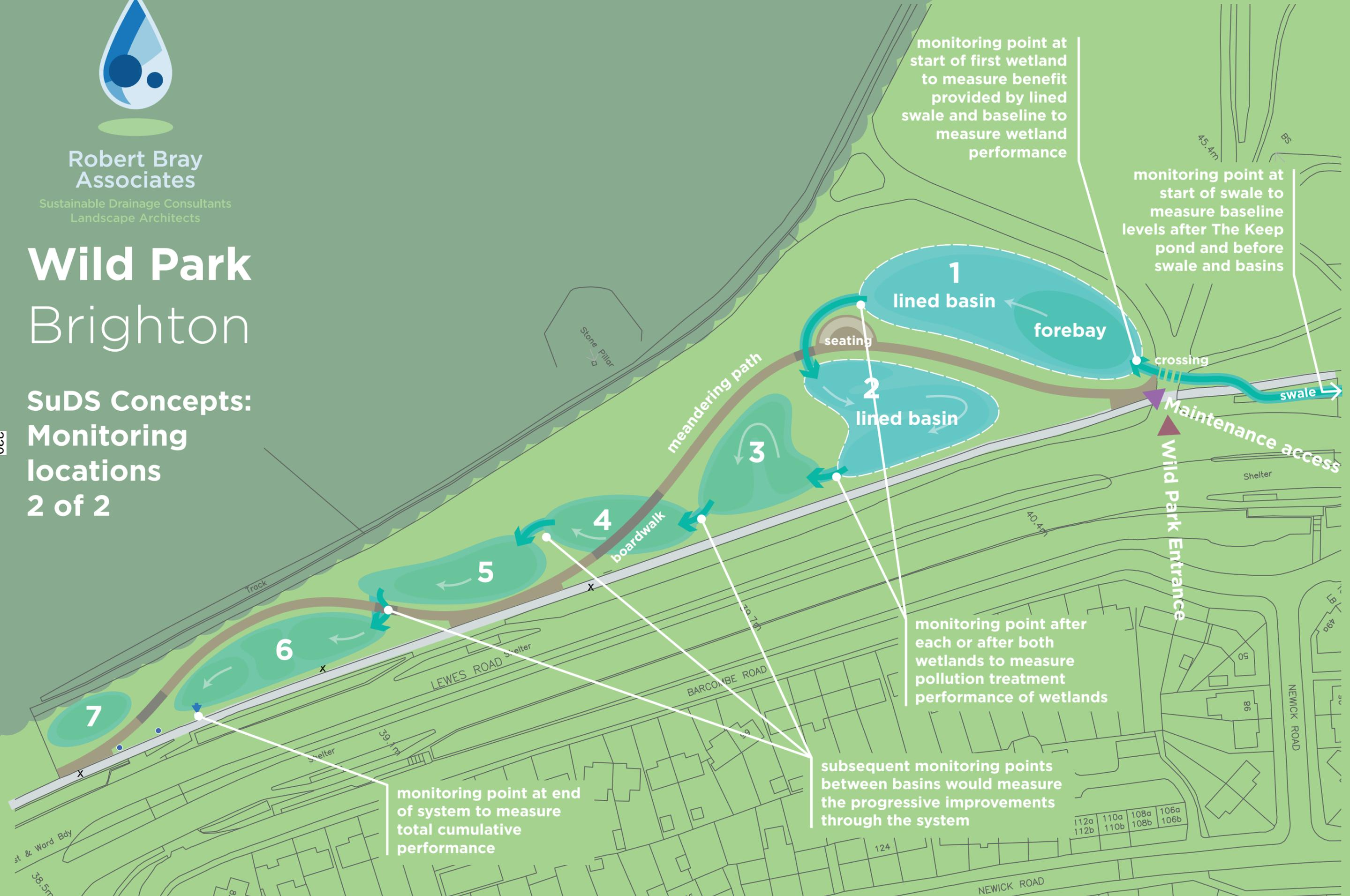
monitoring point at start of first wetland to measure benefit provided by lined swale and baseline to measure wetland performance
